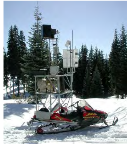
Cloud seeding ground generators
